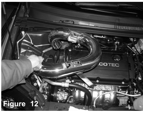
Figure 12 Position the intake tube into the engine bay.
