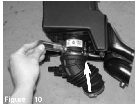
Figure 7 A) With 8mm nut driver, loosen the clamp on throttle body. B) Disconnect the MAF sensor harness.
