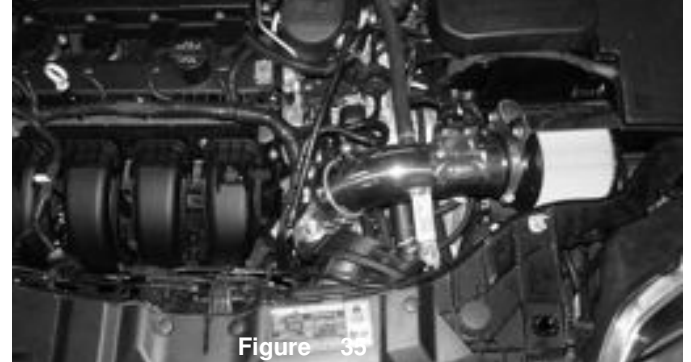
Figure 29 Re-position the filter shield to desired position, make sure that its not touching anything.
