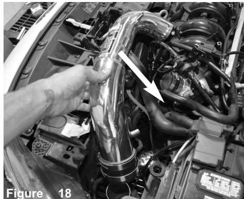
Figure 18 Install upper intake tube assembly and position to lower intake tube and throttle body. Connect the 2 intake tubes together.
