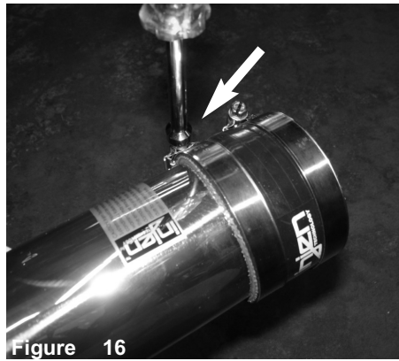
Figure 16 Attach the 2-3/4" straight hose with clamps provided to upper intake tube assembly and tighten on tube only.
