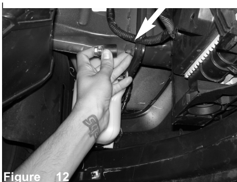
Figure 8 Pull back intake tube from throttle body.
