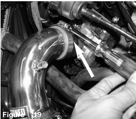
Figure 16 Attach the 2-3/4" straight hose with clamps provided to upper intake tube assembly and tighten on tube only.
