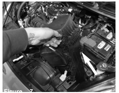
Figure 7 Now lift up and remove the stock air box out of vehicle.
