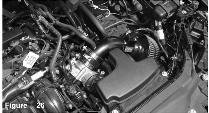
Congratulations! You have just completed the installation of this intake system. Periodically, check the alignment of the intake, normal wear and tear can cause nuts and bolts to come loose. Note: Check clearance and adjust if needed! Failure to check the alignment and adjust the intake can cause damage that will void the warranty. Injen Technology is not responsible for any damages caused by/from improper installation.
