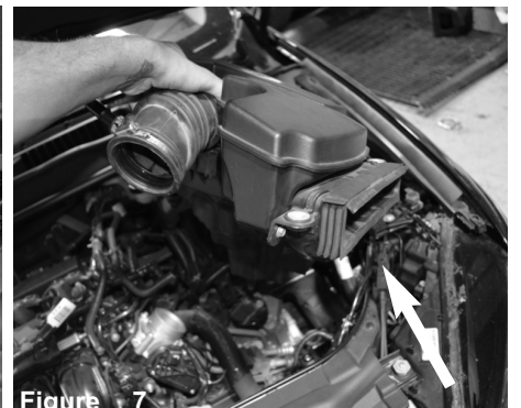
Figure 7 Lift up and remove the air box assembly from the vehicle, make sure the fitting pop out from grommets under neath air box.
