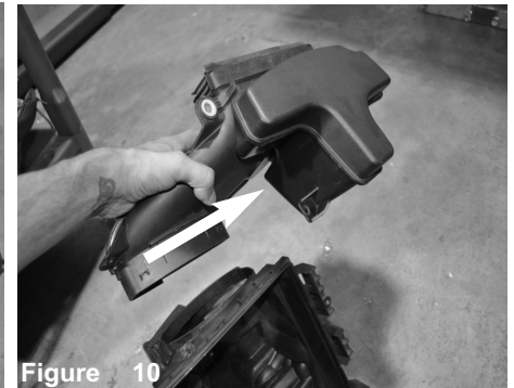
Figure 7 Lift up and remove the air box assembly from the vehicle, make sure the fitting pop out from grommets under neath air box.
