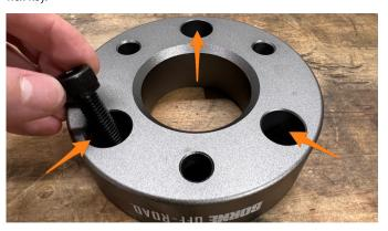
11. Fit the spacer onto the top of the strut. It will only go on in one orientation. Using a 17mm socket, install the spacer using the supplied M10 washers and lock nuts. Use a pry bar against the threads to keep the strut from rotating while tightening the nuts.
