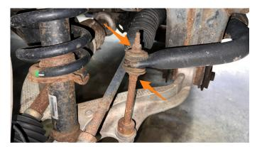
**05.** Using a 21mm wrench, remove the tie rod end nut. Counter-hold the threads using a 10mm socket. Loosely reinstall the nut so that the top of the nut is flush with the end of the threads. Using a hammer, hit the end of the threads to remove the tie rod end from the knuckle. (Image on top right)
