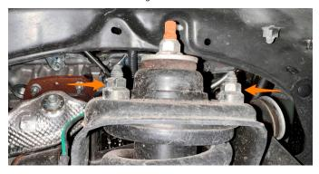
**9.** Push/pry down on the lower control arm (a) until you can get the bottom of the strut (b) out of the mount. Watch the brake line during this step! Make sure not to put any load on it.
