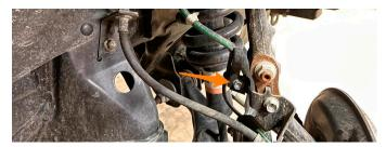
3. Using a trim clip tool, remove the two WSS wire tree clips (a) and unplug the connector (b) on the back of the knuckle and tuck the wire out of the way.
