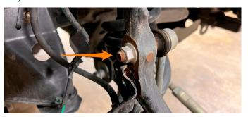
5. Using pliers, remove the cotter pin (a) from the tie rod end castle nut, then use a 19mm socket to loosen the nut (b). Leave the nut partially threaded on for now. Next, using a hammer, hit the knuckle where the blue mark is (c) until the taper pops loose. Leave the nut partially threaded on to keep the knuckle from rotating during the next step.
