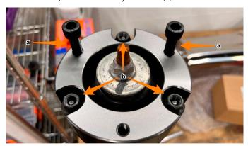
**12.** Using a 14mm socket, fasten the spacer to the strut, counter holding against the bolts with a pry bar as shown. Remove the two M10 bolts once all three nuts are tightened.
