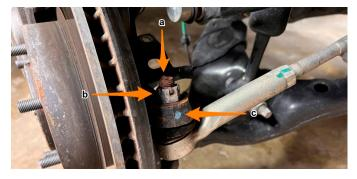
6. Using pliers, remove the cotter pin (a) from the upper ball joint end castle nut, then use a 19mm socket to loosen the nut (b). Leave the nut partially threaded on for now. Using a hammer, hit the knuckle in spot (c) until the taper pops loose. Pry down on the upper control arm and fully remove the nut. You can also fully remove the tie rod end nut at this point.
