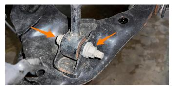
**8.** Use a 14mm socket, remove the three upper strut nuts. The third nut is hidden behind the bushing.
