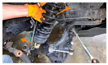
11. Place one of the aluminum spacers on top of the strut as shown and install two of the provided M10 bolts (a) into the spacer. The bolt/hole pattern is purposely not symmetric, so it will only fit in one orientation. Install two of the provided M10 bolts into the spacer, as shown. Partially thread the factory strut nuts (b) onto the threads.
