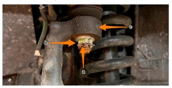
7. Using a 19mm socket and wrench, remove the lower strut bolt and nut.
