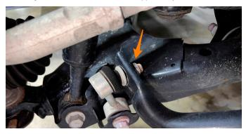
**05.** Remove the cotter pin (a) from the tie rod end castle nut using needle nose pliers, then use a 24mm socket to loosen the nut (b). Leave the nut partially threaded on for now. Hit the knuckle here (c) using a hammer until the taper pops loose. Leave the nut partially threaded on to keep the knuckle from rotating during the next step.
