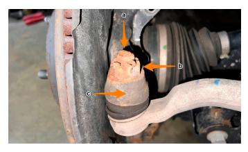
**06.** Using pliers, remove the cotter pin (a) from the upper ball joint end castle nut, then use a 19mm socket to loosen the nut (b). Leave the nut partially threaded on for now. Using a hammer, hit the knuckle in spot (c) until the taper pops loose. Pry down on the upper control arm and fully remove the nut. You can also fully remove the tie rod end nut at this point.
