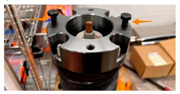
12. Using a 14mm socket and the factory upper strut nuts, fasten the spacer to the strut, counter holding against the bolts with a pry bar as shown. Remove the two M10 bolts once all four nuts are tightened.
