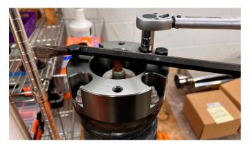
**13.** Reinstall the top end of the strut in the vehicle as shown and partially thread the provided M10 bolts into the top of the strut.
