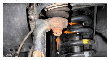
**07.** Tie up the top end of the knuckle to the lower control arm to keep it from hanging on the brake hose.
