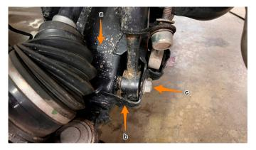
16. Using a 17mm socket, fully tighten the 4 upper strut bolts and untie the knuckle. Next, reinstall the upper control arm ball joint by jacking up on the lower control arm and prying down on the upper control arm (a) until you can get the taper into the knuckle. Keep prying on the upper control arm while tightening the ball joint nut (b) to prevent the taper from spinning.
