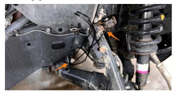
**08.** Using a 22mm socket and wrench, remove the lower strut bolt and nut.
