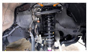
14. Using a metal rod, long extension, or pry bar that fits inside the lower strut bushing (a), rotate the bottom of the strut clockwise (b) until the faces of the bushing line up with the slot in the lower control arm (c). This will require a good amount of force.
