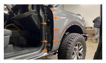
23. Using an 8mm socket, remove the upper screw, then use a 10mm socket to remove the 3 lower screws.
