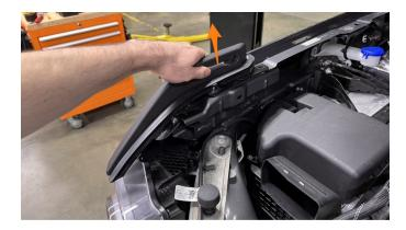
**27.** Using a 10mm socket, remove the screw that was under the bracket.
