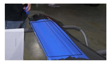
**42.** Coat the unprinted side of the template with a mild adhesive, like the 3M Super 77 spray adhesive or glue stick. Align the marked corner and front side of the template (a) with the mark made in the previous step (b).
