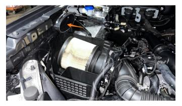
**52.** If using the stock airbox, remove the airbox from the vehicle to better access the bolt right underneath the lip of the adapter.
