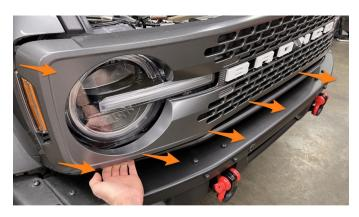
**07.** On the passenger side of the vehicle, rotate the 5 lock levers a ¼ turn toward the wheel. Once the levers are disengaged, remove the fender flare by popping the clips loose, starting at one end and working your way down to release the rest.
