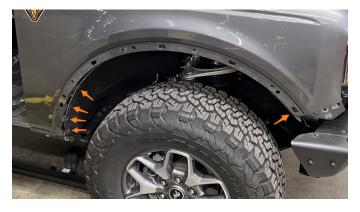
**16.** To remove these clips, use a Phillips head screwdriver to turn the plastic screw about ¼ inch out. Apply just enough force to keep the driver in the head of the screw while turning. If too much pressure is applied, the screw will not thread out.
