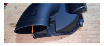
53. Reinstall the stock airbox assembly with the adapter inserted into the silicone coupler. Tighten the worm gear clamp. If using a Mishimoto intake, skip to step 54. Skip to step 55.
