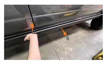
**12.** Next, the passenger side door will need to be removed. Push on the cover (a) and pull the connector (b) out.
