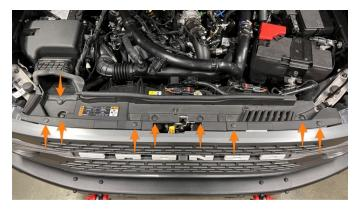
02. Use a trim tool to release the tangs, then remove the air box duct.
