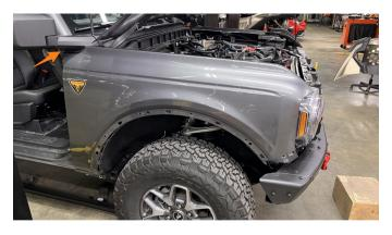
29. If installing the snorkel with a stock intake, the airbox lid must be removed for modification. If installing with a Mishimoto intake, skip to step 39. Use an 8mm socket to loosen the 4 screws until the threads are just visible. The screws do not need to be removed completely. Remove the lid at set aside.
