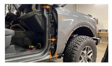
24. Using a 10mm socket, remove the 2 nuts.
