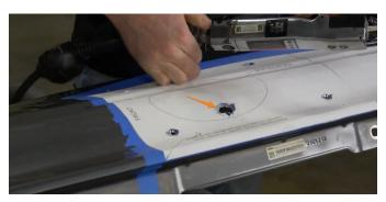
**46.** Starting in the pilot hole, use a body saw to cut out the oval on the template. Once all the holes have been cut out, break all the sharp edges with a file or deburring tool, then remove the template and tape from the fender.
