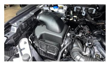
**54.** Install adapter 2 MM2437 into the coupler and onto the Mishimoto airbox. Using a 2.5mm wrench, fasten with the supplied M4 hardware (see parts diagram). Tighten clamp (a).
