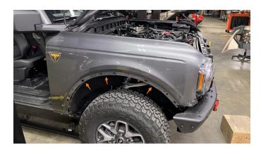
19. Using an 8mm socket, remove the 3 screws.
