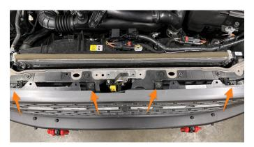
**06.** Remove the grille by starting at one end, popping the clips loose by pulling forward, and working across the bottom of the grille until all the clips are released.
