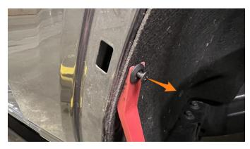
**18.** There are 3 screws located on the fender liner that needs to be removed.
