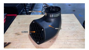
**57.** Install the snorkel head onto the snorkel and use a 10mm socket to tighten the clamp.
