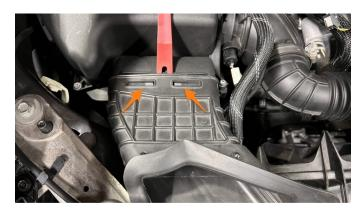
**03.** If equipped, disconnect the front camera by using a pick tool to release the latch, then pull the connector apart. Be careful, this connector is delicate.
