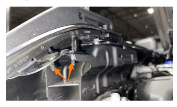
25. Using a 10mm socket, remove the 3 screws.
