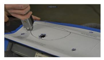
**47.** Lay the snorkel MM2427-01 with an oval tube and brass thread inserts facing up. Place the fender onto the snorkel as shown and line up the drilled holes with the thread inserts on the snorkel. Using a 4mm Allen wrench, fasten the snorkel to the fender with the supplied M6 hardware (see parts diagram).
