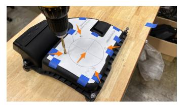
**35.** Firmly hold the airbox lid and use the 4" hole saw to cut the large center hole out. (Image on top right)
