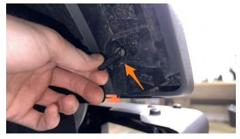
**08.** On the driver side, disengage the first two levers (toward the front) and pop the front of the fender flare loose.
