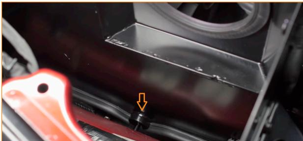
**21.** Secure the airbox mounting bracket with the original bolt. (1x 10mm bolt)
