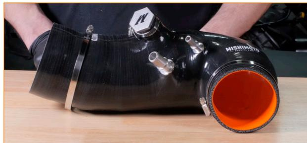
**25.** Install the remaining worm-gear clamps to the induction hose. These clamps are different sizes, so make sure the smaller clamp is installed over the throttle body end of the induction hose. (2x worm-gear clamps)
