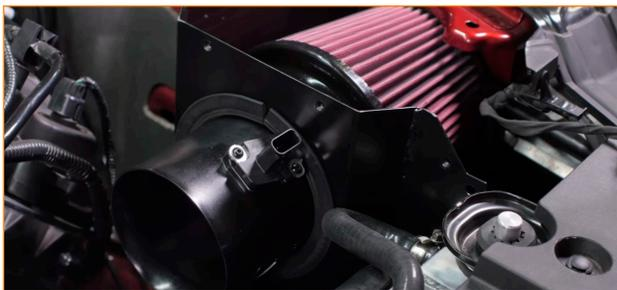
**23.** Lead the MAF wiring around the corner of the airbox and secure it with the integrated tree-clip.
