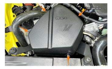
18. Reinstall hose and clip from step 5 if moved out of the way.
