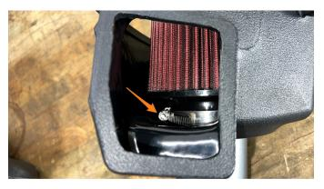
13. Install a 20-32mm worm gear clamp over the small port of coupler 1 then reinstall the CCV fitting into the coupler. Use a 7mm socket to tighten the clamp. Slide a 50-70mm worm gear clamp over the small end of the coupler and a 70-90mm over the large end.
