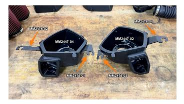
11. Insert the assembled MAF housings into the bottom of the airboxes and push a filter onto each of the MAF housings from the top side.
