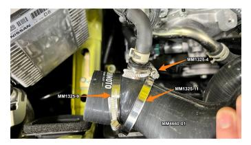
**14.** Install coupler 1 onto the turbo and use a 7mm socket to tighten the clamp on the turbo side.
