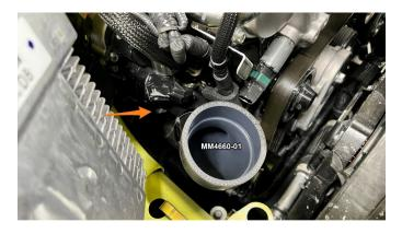
**15.** Plug the connector back into the MAF sensor on the passenger side airbox assembly and install it into the vehicle. Be sure the coupler is fully seated onto the MAF housing flange and then tighten the hose clamp with a 7mm socket.
