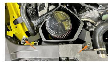
17. Install the passenger side airbox top using the provided O-ring fasteners. Holding the tab, slip the bottom of the O-ring over the lower hook and pull it up over the upper hook. Repeat steps 14-18 for the driver side minus the CCV hose since that side does not have one.
