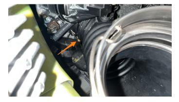
**6.** Using an 8mm socket, loosen the hose clamp on the CCV hose fitting then remove the fitting from the passenger side hose. Both intake hoses can be removed from the vehicle now.
