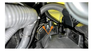
**4.** Unplug the MAF sensor connector from the air box. [Image on next page]
