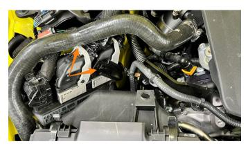
Insert a large pick tool on both sides of the quick connect lock wire to release then, pull the stock air box out.
