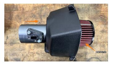
**12.** Using an 8mm socket, tighten the filter hose clamps. They can be accessed through the inlet ducts of the airboxes.
