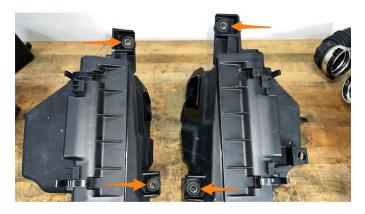
**9.** Using the saved hardware from the previous step, install the MAF sensors into the provided MAF housings.
