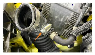
7. Using a 7mm socket, remove the 2 MAF sensor screws from each airbox then pull the 2 sensors out. Save the screws and sensors, they will be reused. (Image on top right)
