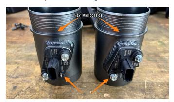
**10.** Using the provided M4 screws and washers, install the brackets to the airbox bottoms as shown. Use a 2.5mm allen wrench to tighten. Install the 4 rubber grommets removed in step 9 into the brackets.
