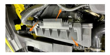
This coolant hose can be unclipped and tucked out of the way for better access to the quick connect fitting in the next step.
