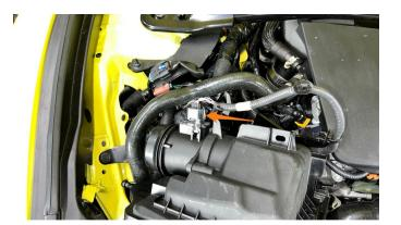
5. Using an 8mm socket, loosen the hose clamp on the intake hose. Repeat steps 1-5 for the driver side.
