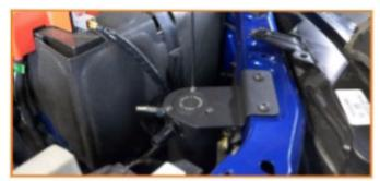
20. Attach the straight hose to the outlet port on the catch can.On late-2021-2023 models, you may trim the rubber hose to length.(1x worm gear clamp)
