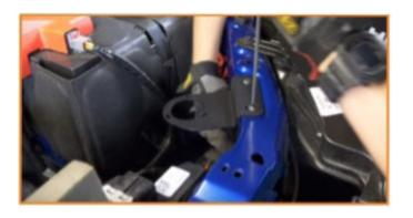
**19.** Attach the bend to the inlet port on the catch can. (1x worm gear clamp)
