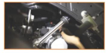
Pull the coolant hose from the clip that holdsit in place.
