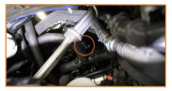
**9.** For late-2021-2023 models, locate the PCV outlet on the intake manifold. Connect the provided catch can hose with the straight
