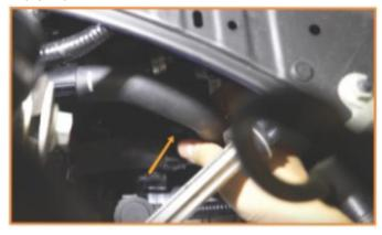
5. Slide the tabs on the PCV quick-disconnects and remove the hose.
