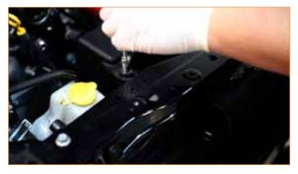
**8.** Tighten down the clamp that holds the induction hose to the throttle body.
